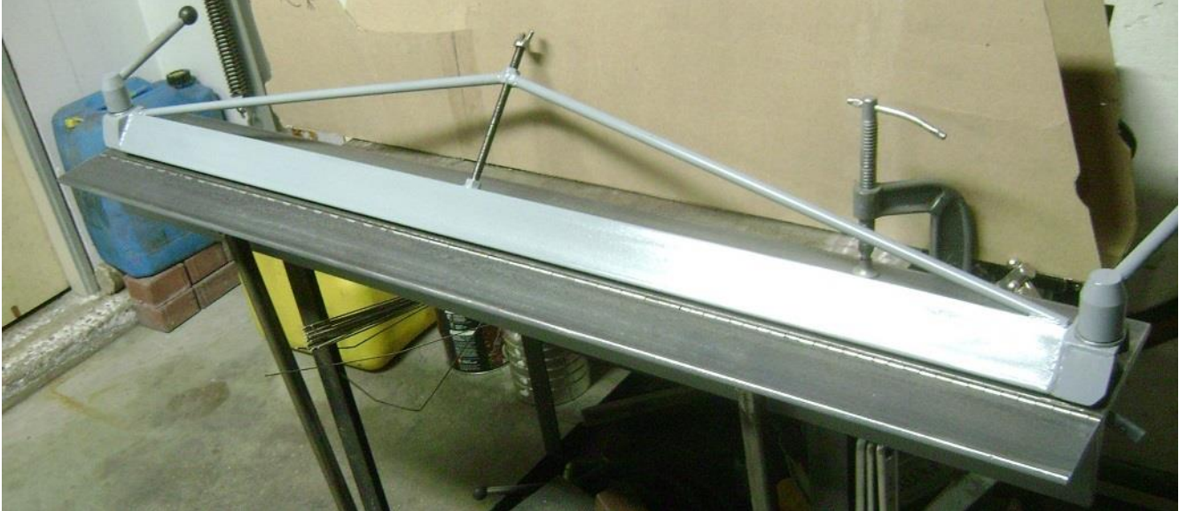
In this month's issue of The Leading Edge, we have a number of helpful tools and hints for aircraft builders from the members of KWRAA. Above is a homemade brake built by Clarence Martens. (Details on Page 2)
