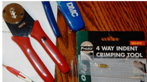
The proper tools make all the difference. Strip the wire and insert it into the pin. Look for wire strands in the inspection hole (special note to Dan!). Put the pin and wire all the way into crimp tool. Squeeze the handle until it doesn't click anymore. Pull it to check and away you go. Push the pin into the connector body and wait for the click. Whoops, wrong hole, then use the \$8 extraction tool to get it right. Better get a high density version as well.
