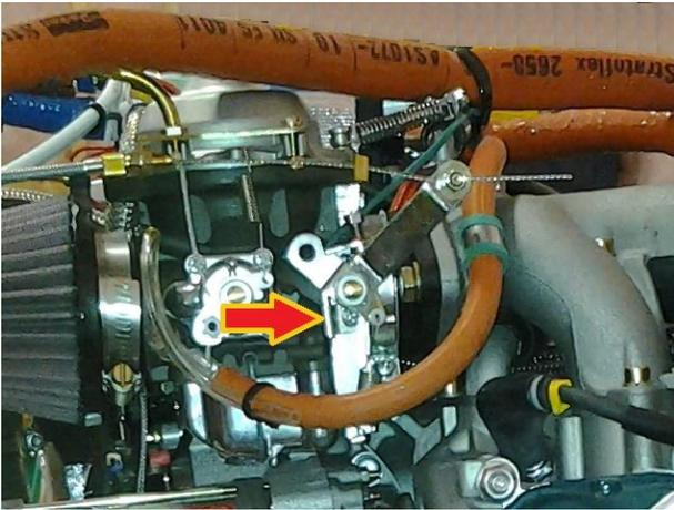
Above you can see the simple clamp holding the thermocouple to the butterfly assembly.
