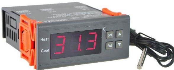
I mounted the thermostats under my panel and the thermocouples on the opposite side of the butterfly as the heating elements. It takes about 30 to 40 seconds to see the rise in temperature on the thermostats, but I assume the butterfly begins to heat in about half that time. I set the thermostats to turn on the carb heat at 10 C and so far have found the system to work well and be trouble free.
