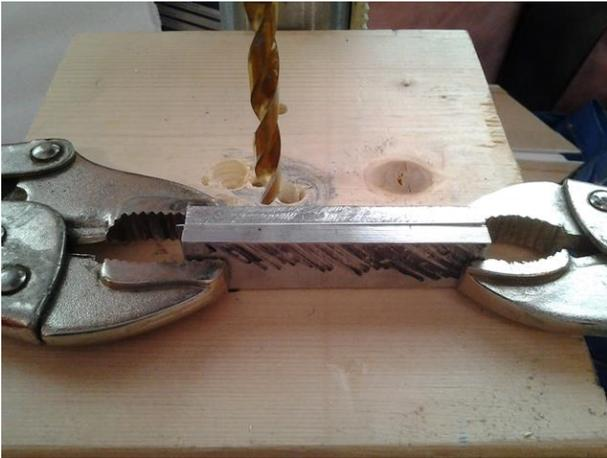
The photo above is to illustrate the process, but it's a good idea to drill the hole in steps to ensure a nicely aligned hole. Start with a 1/8" drill bit then a 3/16" bit then finally the 1/4" bit to get the final size.
