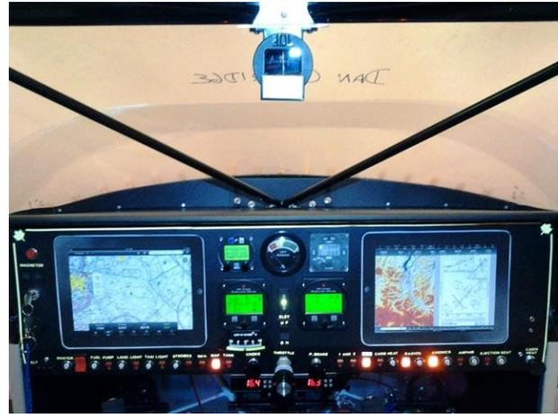
Above you can see the thermostats mounted just below the throttle and displaying the current carb temperature.
