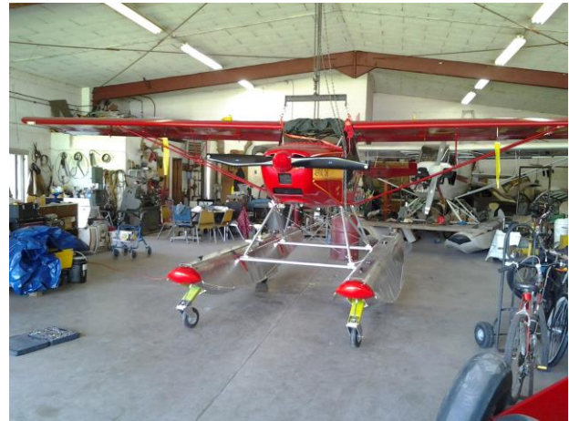
As we slid the floats under the airframe and fastened them, it looked like they really belonged under there
