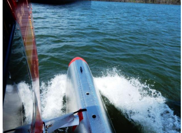
Taxiing in displacement mode, the plane sits quite high on the water with these amphibious Zenair floats
