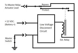
Switching the circuit to bypass during starting will eliminate this problem, but that defeats the purpose of having a system that works automatically, so a modification is in order.
