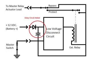
This option would likely require a bit of trial and error to find the right value of capacitor to keep the circuit on long enough to prevent the low voltage circuit from oscillating like it is now without oversizing it, which could prevent it from reacting as it should to protect the battery.
