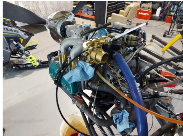
Injector blocks and throttle bodies installed. Ignition modules have been lowered to clear the linkage
