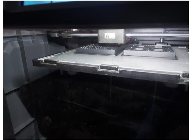
3D printing brackets for fuel pumps
