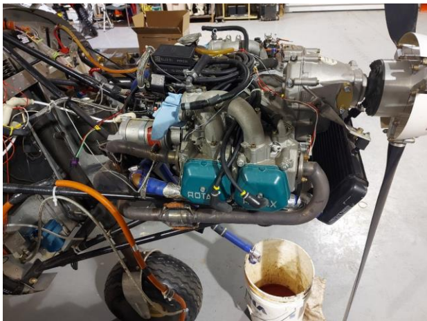
Rotax 912 ULS with the carbs removed
