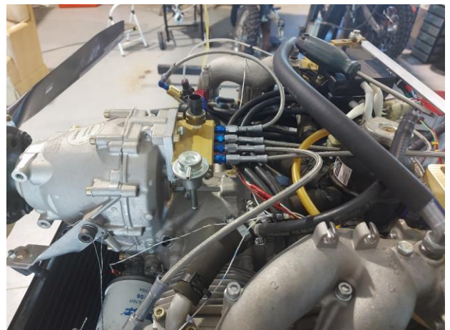
Fuel block and lines to injectors
