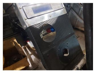
Perfect 2 1/4" diameter hole. The only chips to clean up were from drilling the pilot hole.
