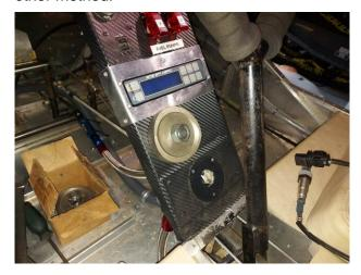
A fuel line was in the way, so I had to temporarily remove the fuel selector valve. Punch has done its work and is ready to be removed.
