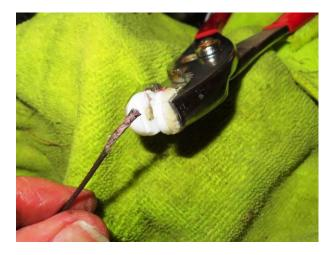
**Step 6:** Carefully apply Loctite Permanent Thread locker and work it into cable end using the pliers. Keep pulling the cable through the pliers until it is smooth.
