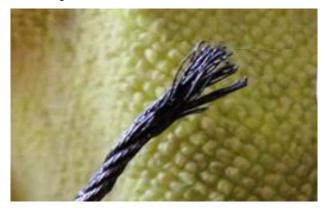
Last time this happened was on the dock in Sault Ste. Marie, several hours from home. Like many amateur-built aircraft mine also has other similar cable controls, including some for my gear retraction and rudder controls. After 12 years of fighting with this problem, I thought there must be a solution. The plan would be to trim the cable ends, and seal them with cyanoacrylate (crazy) glue and thread locker using some special "slippy" pliers that I made.
