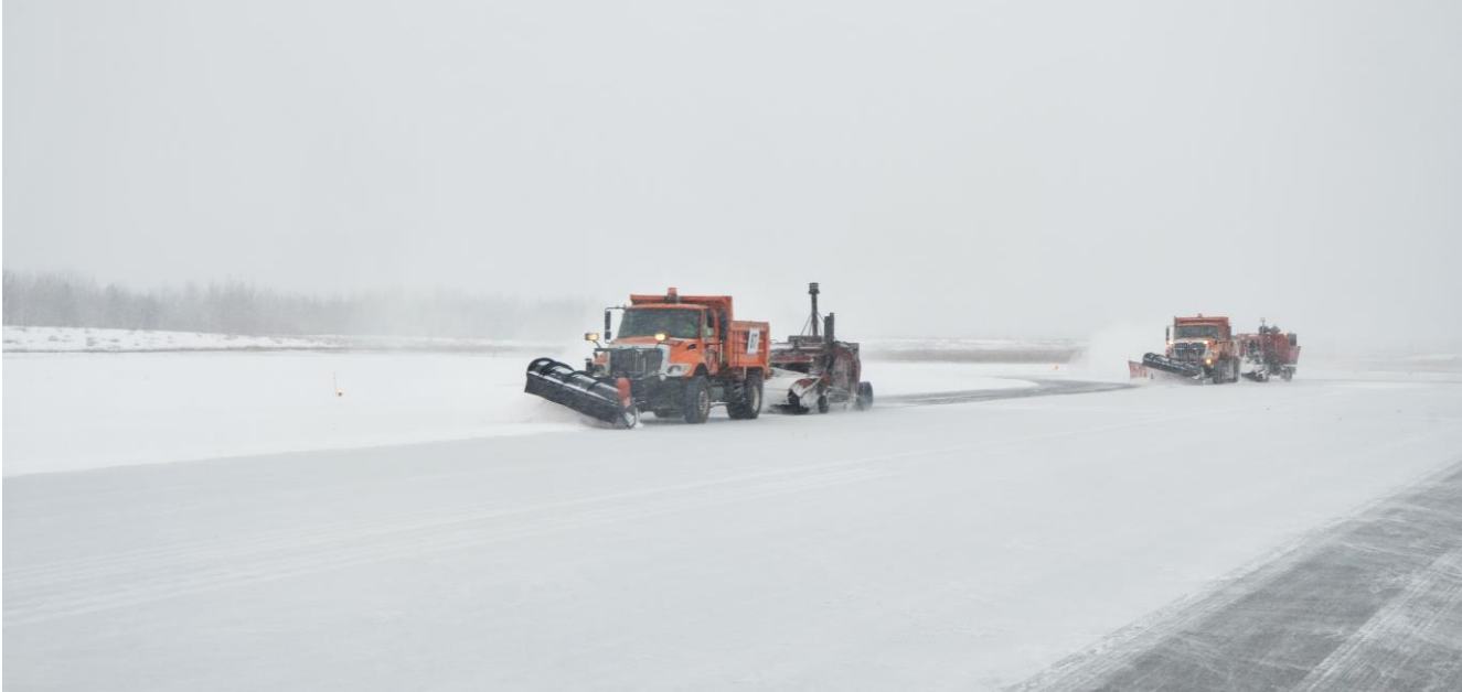
Snow Plow/Sweeper combination vehicles keeping the runways clear at CYSB. Similar rigs are used at most airports in Canada that handle commercial air traffic, including CYKF.
