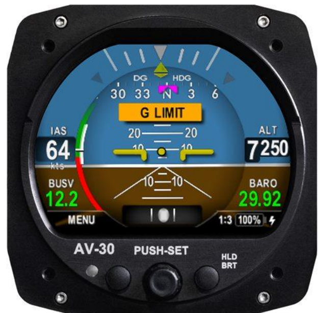
The 3 1/8 inch AV-30 is another option for controlling the tailBeaconX. Its larger format allows it to operate as a primary flight display and has additional features over the AV-20 including digital precision attitude and directional gyro customizable displays.
