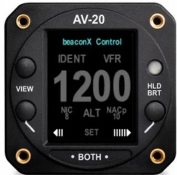
The AV-20-S is a 2 ¼ inch FAA-approved Multi-function Display that can control the tailBeaconX and provide a number of other useful functions.
