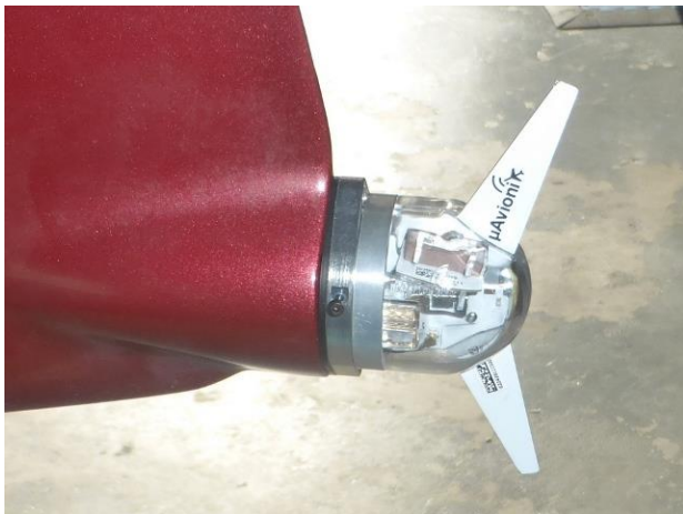
tailBeaconX replaces an existing tail light to provide 1090 ES ADS-B OUT for satellite and ground stations
