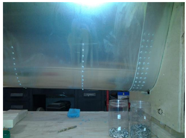
The joined sheets are clearly visible in this photo and the excess zinc chromate has been wiped off.
