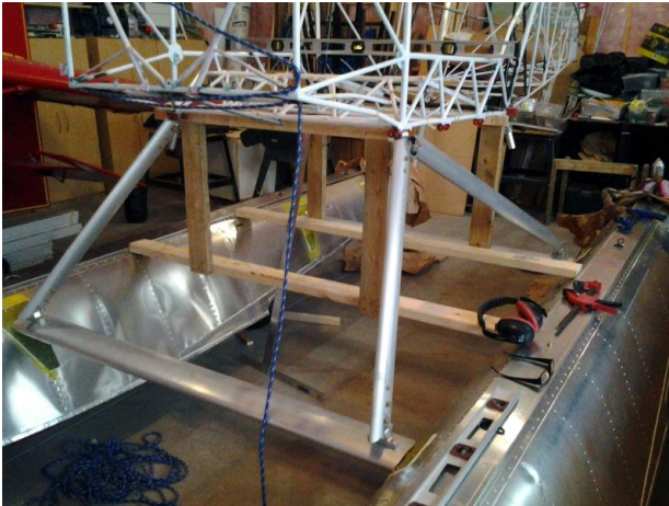
The weight of the fuselage held the whole assembly from moving on the wooden jig I used for rigging.
