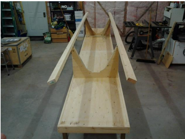
The first challenge is building a 16 foot long work table to cradle the floats as you start construction.
