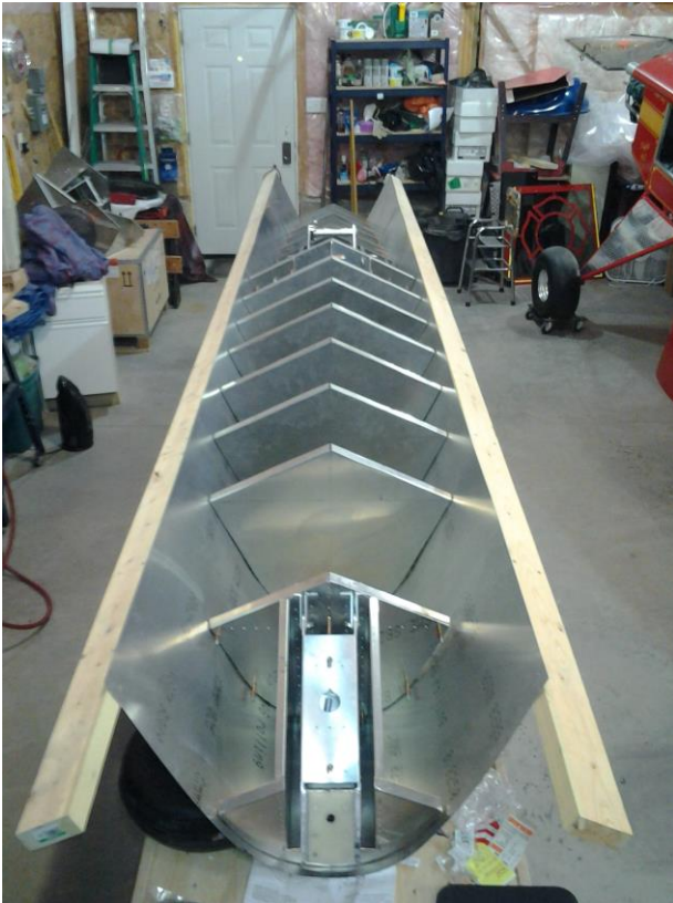
Once the bulkheads are fastened into position with clecoes the float starts to take on a familiar shape.
