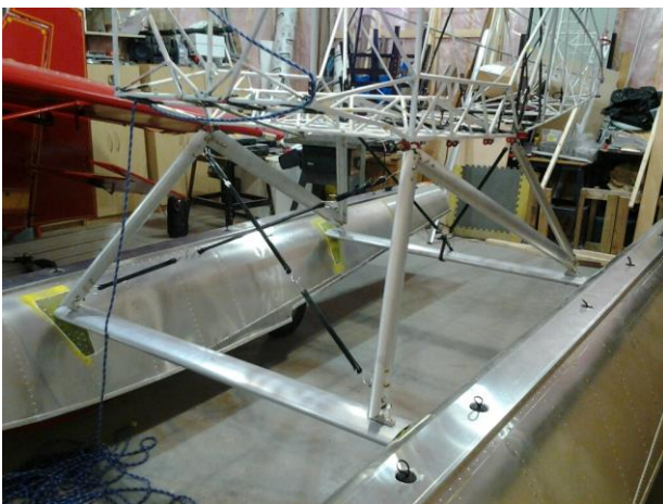
Well cut and nicely fit spreaders and supports make for a clean installation and lower drag. The bungees were used to temporarily hold things under tension. Wire bracing and turnbuckles will be used during the final rigging on the Highlander.
