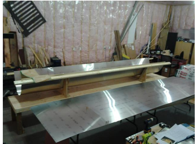
At 15' long, the Zenair 1450# floats require a 3' long piece be fastened to a standard 4x12' sheet of 6061.
