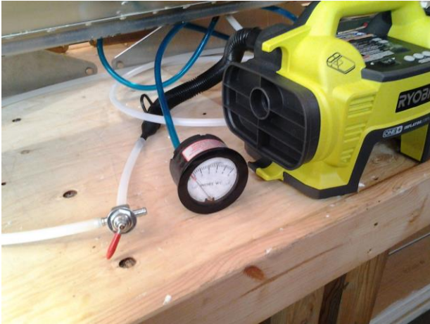
A portable inflator, low pressure gauge and small valve helped to control the leak testing process.
