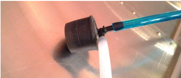
A portable inflator, low pressure gauge and small valve helped to control the leak testing process.
