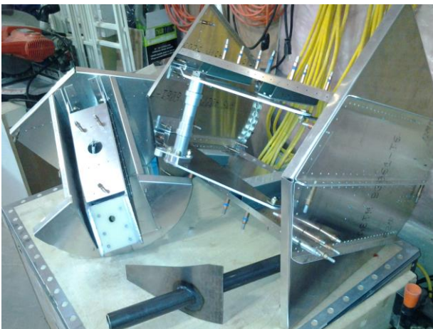
The wheel assemblies can only be fastened into position after the internal extrusions and braces are drilled, aligned, glued, riveted and sealed in place.
