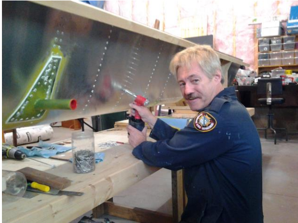
A pneumatic riveter and some occasional assistance from the better half are priceless when float building.
