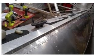
I then made new trim strips and clamped them in place with vice grips, spring clamps and sealant. Sikoflex cures in about 4 to 6 hours allowing me to move on to the next piece.
