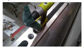
I mounted a Scotchbrite pad on a drill mandrel and used that to clean and polish the inside of the cups and then used a flat piece of Scotchbrite and some cleaner/de-greaser to clean the rubber plugs. I was very pleased with the resulting smooth and clean surfaces, which should restore the seals to like-new condition.
