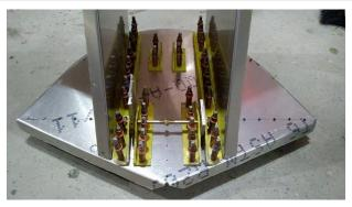
Satisfied with the result, I began assembling the parts I had made and added the extrusions back into the assemblies. Everything was done with clecoes first, of course, since final assembly would require the addition of adhesive sealant for waterproofing.
