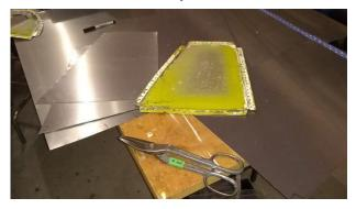
By hammering some of the aluminum bulkheads and skins out flat, I was able to trace them and lay out some of the critical hole positions in the new parts I was making.
