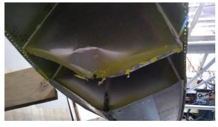
Once the lower skins were removed, the damage to the bulkheads was more apparent, but still what I expected to see.
