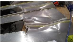
The new and original skins are shown here for comparison. I only replaced the bent section, but did a triple row of rivets and overlapped the bottom skins at a bulkhead to ensure a very tight and secure seal.
