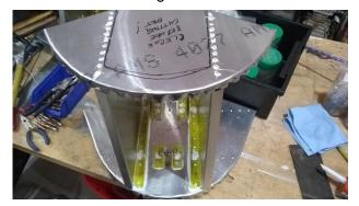
Once everything was cleaned up and the new aluminum roughed up a bit, I added the sealant to each joint and began final assembly.
