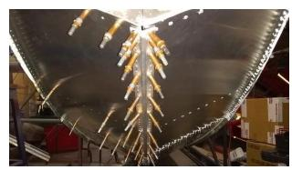
I then test fit new pieces of keel extrusion and drilled half a bazillion holes to mount them temporarily with clecoes. Next, I drilled another half a bazillion holes out the bottom skins to match the holes that take 3/32" squeezed rivets that join the bottom skins to the side skins. I then disassembled everything and deburred all one bazillion holes.
