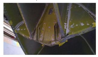
Drilling out the pulled rivets was the method of choice to gain access to the sealant that still held everything together. I made a small ruler-like tool with a sharpened end that I used to cut
