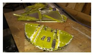
Many of the rivets inside are structural stainless steel rivets and presented quite the challenge to remove. I found that the bits of mandrel left inside some of them meant that I was replacing drill bits quite often and sometimes could not get the drill bit to align with the centre of the rivet.
