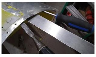
I removed the upper walkway the same way. It had to be removed in order to gain access to the top rivets in each bulkhead to be replaced.
