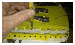
I found that driving the mandrel bit out with a small centre punch worked well and made the drilling job easier. Applying a drop of cutting oil to the tip of the drill bit made the job easier and faster as well as reducing my dulled-out drill bit to rivet ratio substantially.
