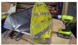
The flattened bulkhead served nicely to align all of the critical holes and then many of the final holes could be back-drilled through the extrusion to ensure perfect alignment on the new bulkheads.
