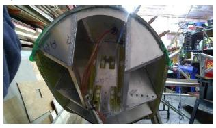
I trial fit the wheel bulkhead assemblies into the floats,
