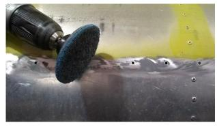
Removal of the sealant on exposed surfaces was hastened by the use of a small drill-mounted Scotchbrite pad. I just had to hold on tight and develop a knack for keeping the pad from running away down the surface beyond where I wanted it to go.
