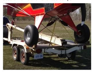
This works well for my plane, given the firm springs on the trailer itself, which are likely a little too firm to strap the fuselage to the trailer using a solid support. I have seen photos of a Kitfox that had been strapped over the fuselage solidly to the trailer and it severely bent the fuselage longerons at the strap when subjected to road travel. I like to let the plane float on its own suspension with straps limiting the upward travel while securing it to the trailer.
