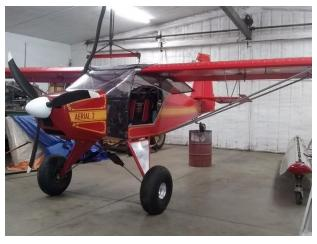
I use an empty 45 gallon drum to support the tail at the correct angle for the floats.
