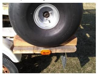
The deck for the mains is made from three 2x8's that are seven feet long and secured with bolts through the trailer's steel frame.
