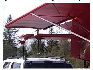
To off-load the plane, simply reverse the steps. Remove the straps, clamps and rear chocks, install the ramps, use the drill to loosen the winch cable and slowly walk the plane down the ramps using the winch and drill as a brake.
