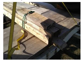
The tailwheel ramp is then fastened to the centre U-shaped rail and the ramp for the mains is strapped to the trailer's steel cross beams just ahead of the wooden deck.
