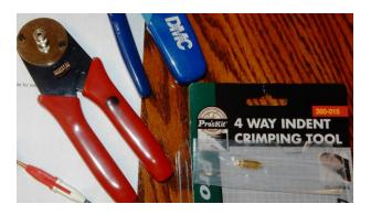
The proper tools make all the difference. Strip the wire and insert it into the pin. Look for wire strands in the inspection hole (special note to Dan!). Put the pin and wire all the way into crimp tool. Squeeze the handle until it doesn't click anymore. Pull it to check and away you go. Push the pin into the connector body and wait for the click. Whoops, wrong hole, then use the \$8 extraction tool to get it right. Better get a high density version as well.
