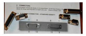
But, not all D connectors are created equal. It is important to match parts, using high quality solid pins and sockets with matching bodies. Luckily, there is a MIL-SPEC governing these and Aircraft Spruce (ACS) has the right parts, mostly.
