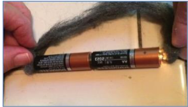
Fine steel wool and two AA batteries used as a fire starter. (Source: Before It's News.com)
