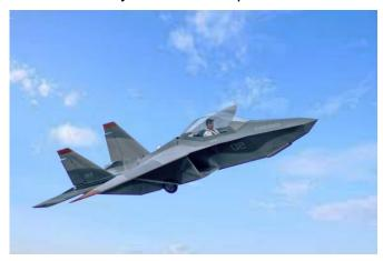
Originally designed to operate using a Rotax 503 with 50-65 hp., the SF-1 has an empty weight of roughly 445 lb. The very first engine used for testing only developed 45 hp yet achieved 100-mph cruise speed. With a Rotax 503, wing loading was less than 4 lb./sf! Google "Archon SF-1" for videos.
