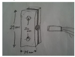
First we needed to make a couple of aluminum clamps that would hold the heating elements against the carbs.
