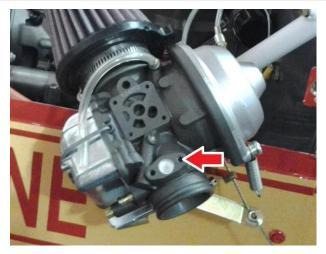
Be careful not to drill too deep as to go all the way through the material. Use a drill collar or drill press set to only go 7/16 inch deep. Tap the holes for a #8 machine screw.
