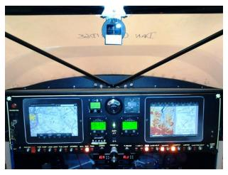
Above you can see the thermostats mounted just below the throttle and displaying the current carb temperature.
