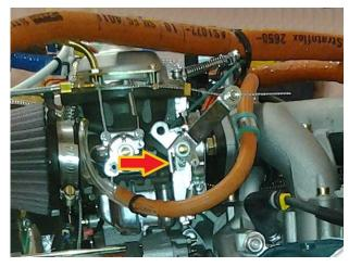
Above you can see the simple clamp holding the thermocouple to the butterfly assembly.
