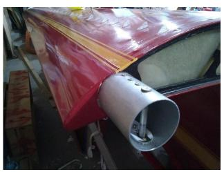
I waited several hours between sections to allow the foam to set up. Once completed, I trimmed off any excess that had seeped out and installed coloured vinyl over the entire length of the leading edge to match the paint on the plane. I then trimmed out the installation with a little reflective gold vinyl like I have on the rest of the plane to make the installation look like it has always been there. I was very happy with the
