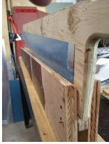
In the end, I found that I had to hammer the upper form into the lower one with a rubber mallet while applying significant force from my body weight to get the aluminum to conform to the curve within the tight form I had made. But, it did work! I was able to reproduce the curve to make enough pieces to form the new leading edge.
