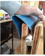
To get the droop, I had to reposition the upper form and using a long dowel, re-drove the upper form into the lower one with the aluminum off to one side. The trick here is getting the curve consistent through multiple pieces. But careful planning and measurement paid off.
