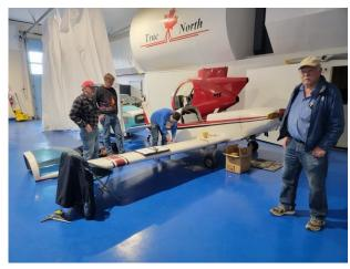
One of the donated props is a Rand KR-2 fiberglass over foam and wood aircraft that flew here from Vancouver to be donated by the owner. The KR-2 is a 165mph two-seater that is VW powered and has a wooden propeller. The agreement was that it would never fly again, so we set about modifying it into a teaching aid.
