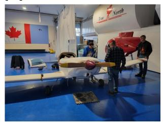
The guys mounted the second wing and refined the folding mechanism.
