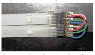
The picture above shows two strips with one tri-colour LED module and 3 resistors in each, these resistors correspond to the different colour strings. The positive voltage is connected to the "+" terminal, coupling to the colour strings "R", "G" & "B". Each of these resistors is different, to adjust the current for equal brightness to be able to see "white" with 12V applied. The supplied remote control has specific voltages programmed for each of the RGB LEDs to select predetermined colours.
