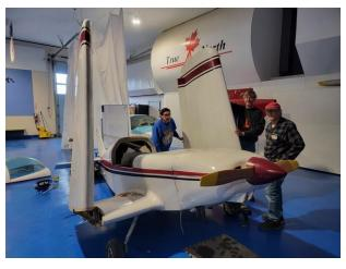
In order to fold up to, and beyond, 90 degrees meant that the upper wing surface had to be carved out to allow it to fold into itself. This left a bit of a gap, which will be covered with a thin removable strip when on display.
