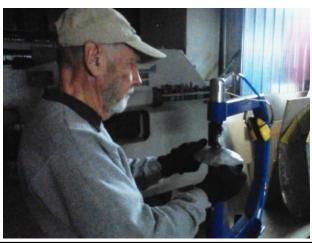
As the fairing started to take on the basic shape required, he inspected it to determine what further working of the material would be required to get it smoothed out.
