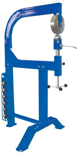
This is what the English Wheel from Princess Auto looks like. Gary's is slightly different in construction, but the working mechanism of a flat wheel and domed wheel is the same. The rack of different sized domed wheels on the left side of the stand allows for different radius bends to be worked on the wheels.
