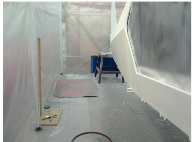
Here is the fuselage primed and you can see a small wood stand with a 4" nail near the top that I made to hold the spray gun. It's true that 90% of the job is preparation.
