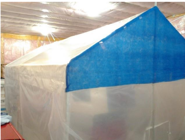
Here is how it looked completely assembled and showing the large air intake area. The blue quilt batting was on sale for only 99 cents a yard. (Reg. $2.99/yd.)
