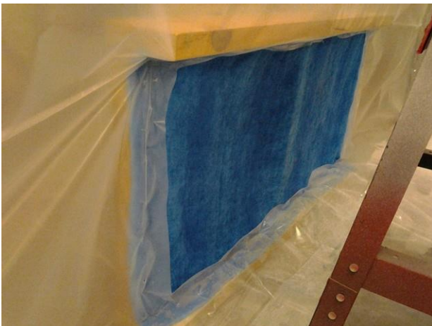
I used quilt batting for a pre-filter and a 2x4 frame to hold the fans and filters in place. Stapling the plastic to the frame made a quick and simple seal.
