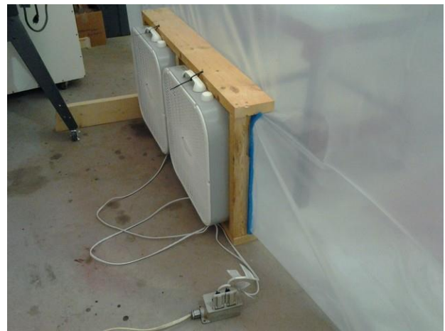
Here you can see the outlet side of the fan assembly. Even after several coats of paint, the fans barely had a perceptible amount of pink colour from the red overspray.
