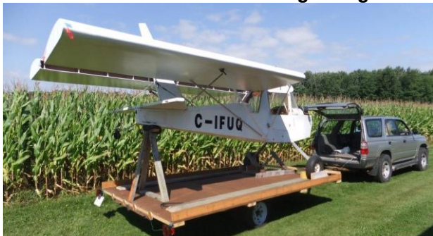
Everyone was checking out the folding wing conversion on Mike Thorpe's HighMax ultralight
