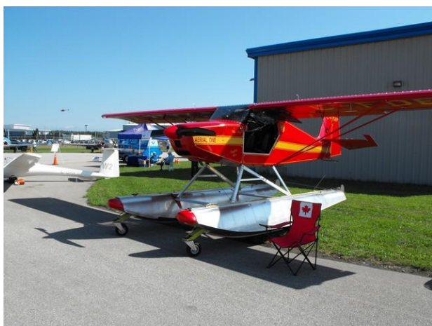
My Highlander got a little sun this year. We couldn't get it into the Cadet building with the floats on it. With the wings folded, it would have tipped over backwards because the mains are so far back. This wasn't an issue when it was a taildragger on bush gear.
