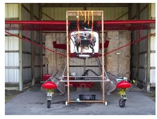
With the engine safely cradled in the straps, I removed the engine mount and had it checked for cracks. The powder coat had to be burned off to get a closer look. Surprisingly, there was no crack! Only the powder coat showed a cracked surface, so to be safe the rest of the major joints were checked also.
