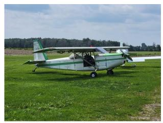
Ivan's unique hybrid aircraft has an unusual mix of parts from different aircraft and a profile that his wife calls the drumstick plane. Its unique construction has a chromoly frame like a rag and tube, but also has an aluminum skin like a typical Cessna. It has some features like a Bird Dog, but others that are very unique. I'm partial to the gull wing doors like my Highlander has.
